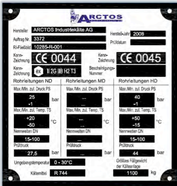
Manufacturer's nameplates for both refrigerant circulation of the CO 2 / propene-cascade refrigeration system
