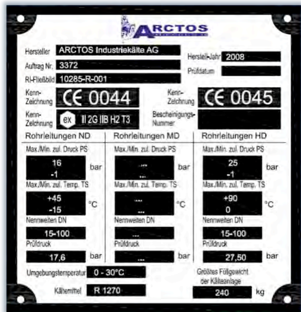
Manufacturer's nameplates for both refrigerant circulation of the CO 2 / propene-cascade refrigeration system
